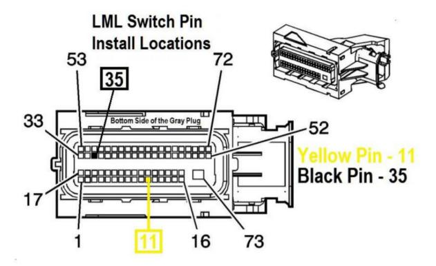
LML DSP Switch Installation
