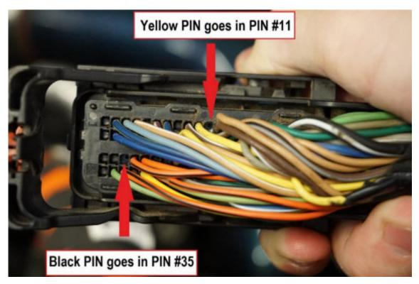
LML DSP Switch Installation
