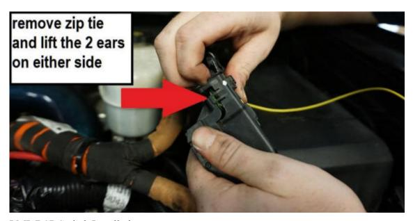
LML DSP Switch Installation
